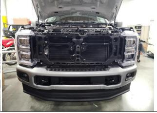
Remove the 2x 10mm bolts form the top of the DS headlight and the 13mm from the bottom by accessing it from the fender well. Pull the headlight out and remove the electrical connectors on the back. Find the included backlight wiring harness and locate the scotchlok connector. For trucks with stock LED headlights, place the scotchlok connector around the wire coming from Pin 8. For trucks with halogen bulbs, place the scotchlok around the Pin 2 wire of the two-pin connector.
