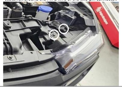
4. Route the wire lead to the LP4s. Using a flathead screwdriver, remove the green cover on the front of the Deutsch connector of the main harness. Insert the wire into the #3 position until it clicks into place and replace the cover. Repeat for the other light. Tie all excess wire into a service loop and reinstall all removed components.
