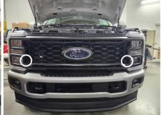
2. Carefully pull the front grill out disengaging the plastic clips. Remove the electrical connector and water line from the grill to free it. To remove the water line, remove the small black plastic ring and pull.
